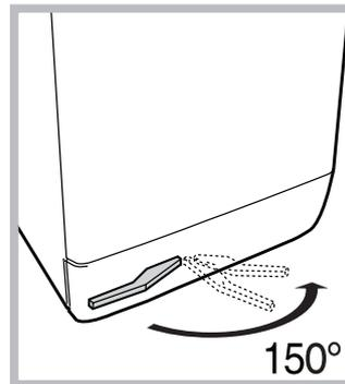
If your washing machine is equipped with a special set of retractable wheels you can easily move it. To lower the wheels and thus move the appliance effortlessly, just pull the lever, situated on the left-hand side beneath the base. Once the
