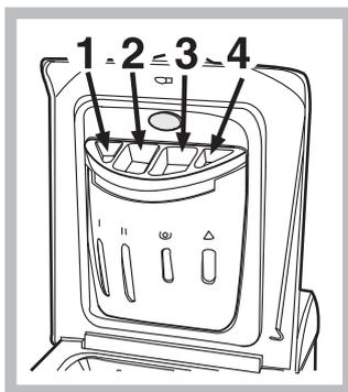
To run the bleach cycle on its own, pour the bleach into compartment 4, set the "Rinse" programme and activate the "Stain removal" programme. To bleach during a wash cycle, pour in the detergent and any fabric softener you wish to use, set the desired wash cycle and enable the "Stain removal" function.
