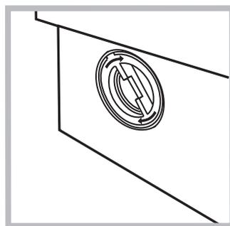
1. remove the plinth at the bottom on the front side of the washing machine by pulling from the side with your hands (*see figure*);
